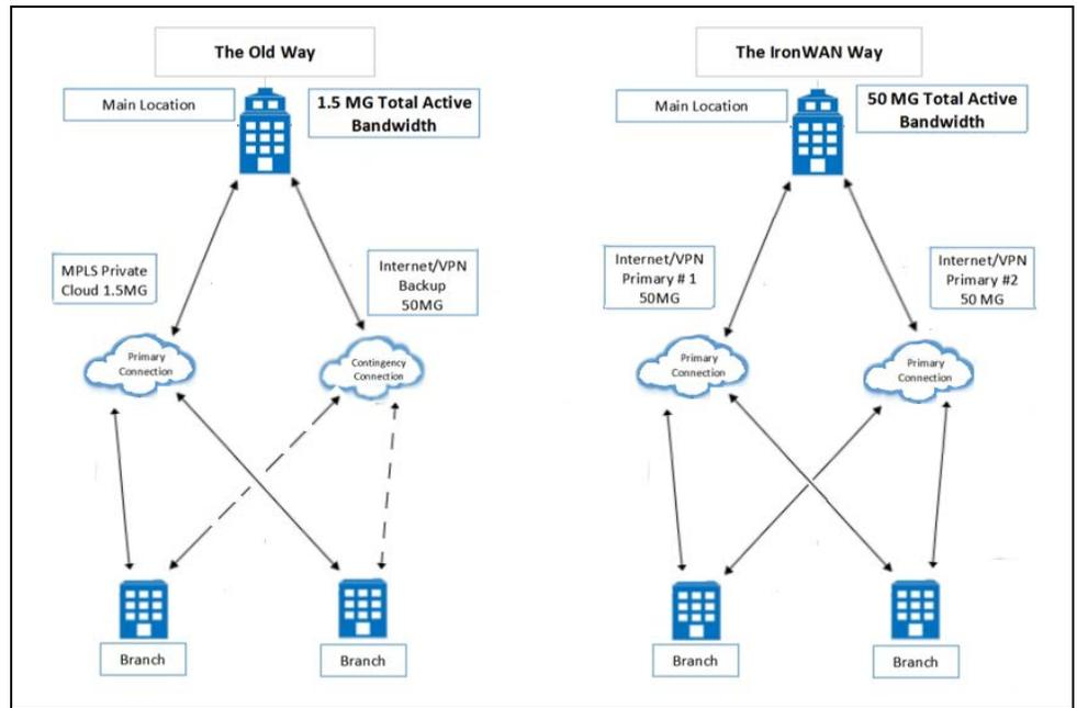
aggregated amount of bandwidth, at all times. This eliminates the need to over-provision expensive MPLS bandwidth to accommodate traffic spikes and eliminates unused bandwidth that is being licensed only as a back-up failover link. Policies can also be written to grant your most critical applications the highest network priority to ensure the low packet loss and latency to keep priority packets from dropping or degrading.
